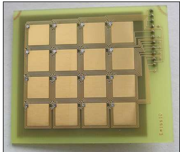
Figure 1. – The sensor card before black painting
