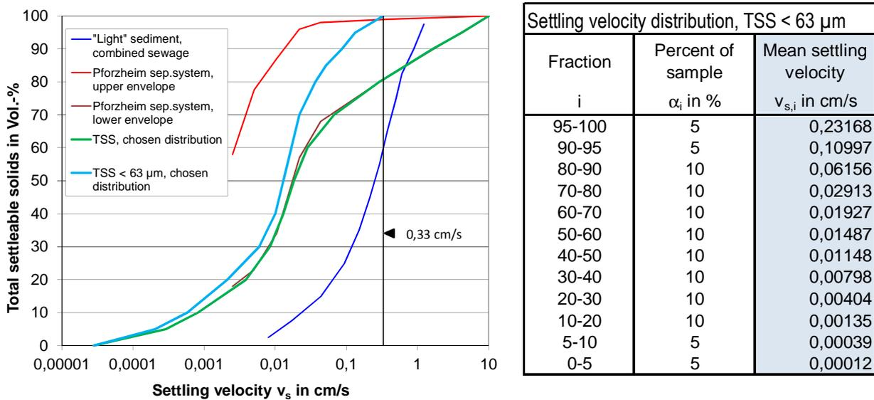
Figure 3 : Distribution of settling velocity  $v_s$  for very fine TSS in surface runoff of separate systems, Weiss (2014b)
