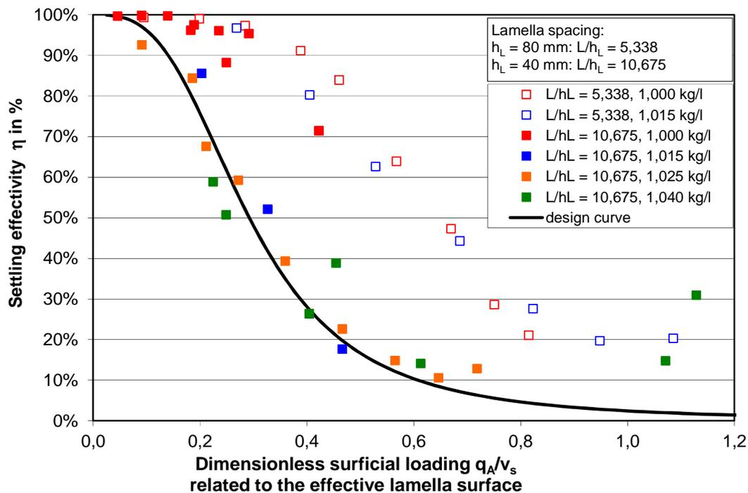
Figure 2 : Dimensionless results of model tests for 40 mm and 80 mm lamella spacing (see Kemper et al. 2014b)
