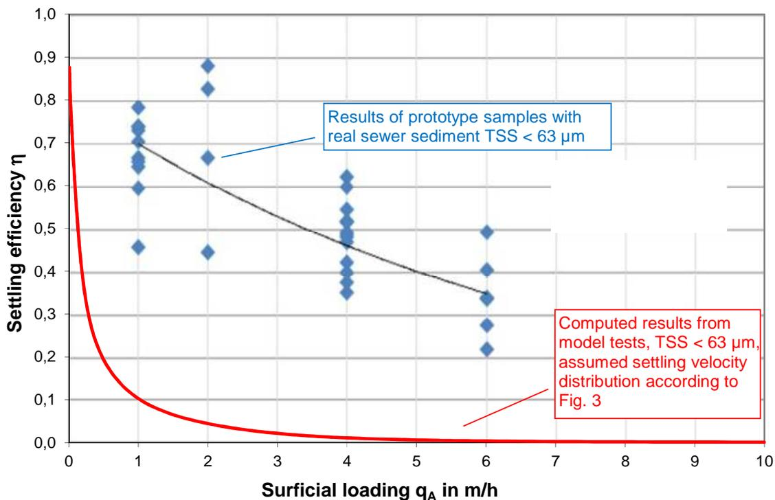
Figure 4: Comparison of measured settling efficiencies of real sewer sediment (TSS < 63  $\mu\text{m}$ ) to computed values from model tests
