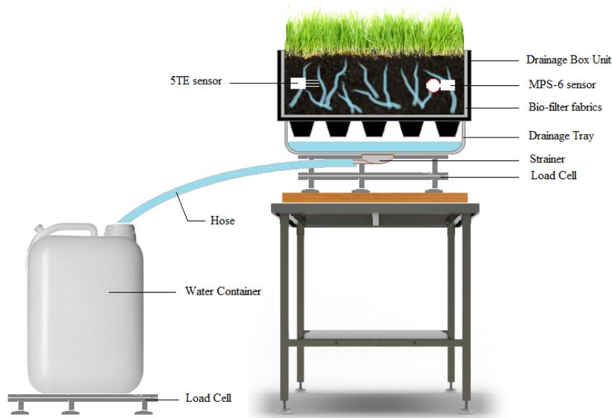
Figure 1. Weighing lysimeter and water container
