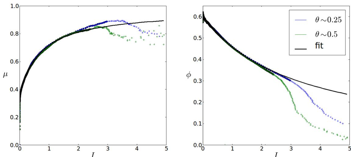
Figure 3: The particle shear to normal stress ratio  $\mu$  and the solid volume fraction  $\phi$  are plotted as functions of the inertial number. The two parts shows different behavior with a clear trend in the dense flow, and a more chaotic one in the fluid-dominated part. The dense part can be fitted by a law of type  $\mu(I)/\phi(I)$  (8,9) with phenomenological constants  $\mu_1 = 0.35$ ,  $\mu_2 = 0.97$ ,  $I_0 = 0.69$ ,  $\phi_m = 0.6$  and  $a = 0.31$  (fit).
