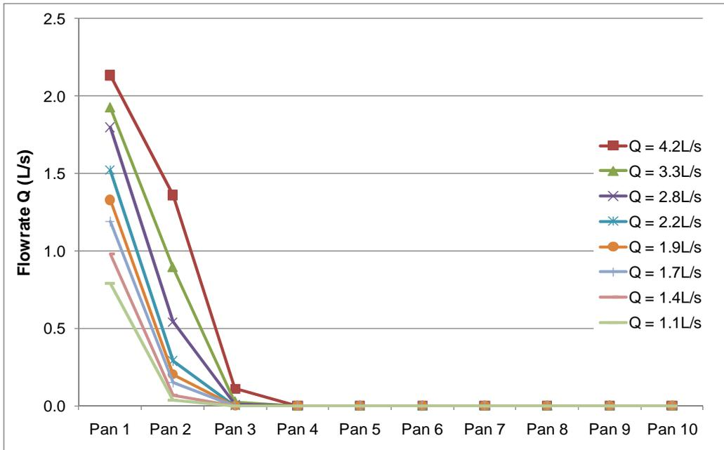
Figure 6. Impervius Concrete Block Pavers 5% Slope
