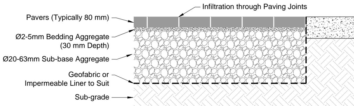
Figure 1. Typical PICP Paving Bed Cross Section
