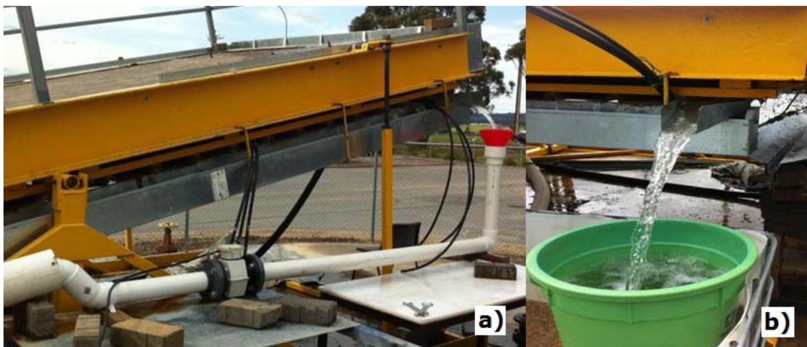
Figure 4. (a) Measuring Individual Pan Flowrates using EMF; (b) Volumetric Method
