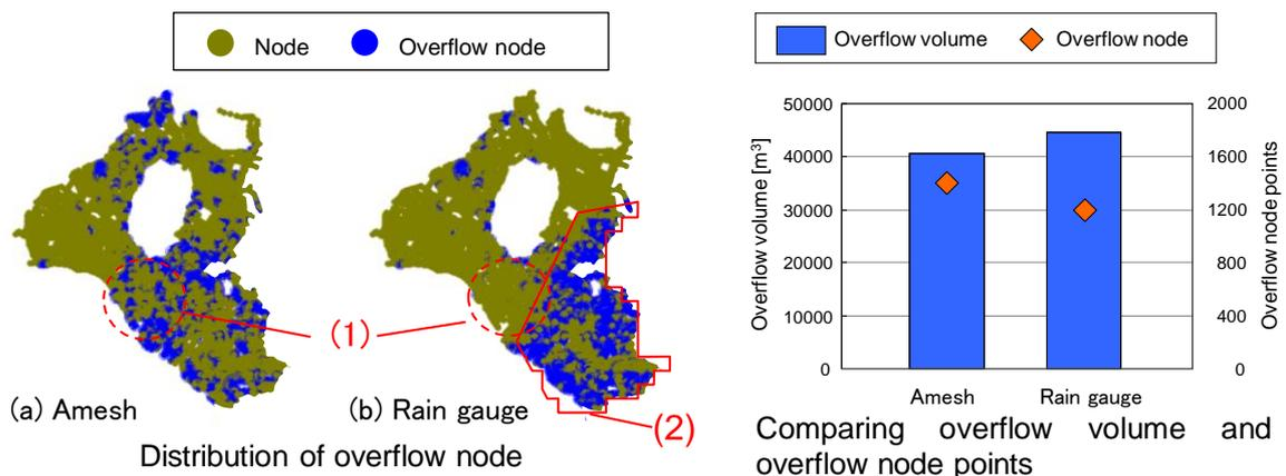
Fig. 1 Simulation of inundation situation. Distribution of overflow (left) and comparing overflow volume and overflow node points (right). (1) Results by using Amesh radar could express local inundations. (2) Results by using rain gauge data was reflect compartmented rainfall information
