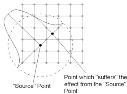
Fig. 4: Delocalization of the damage variable
