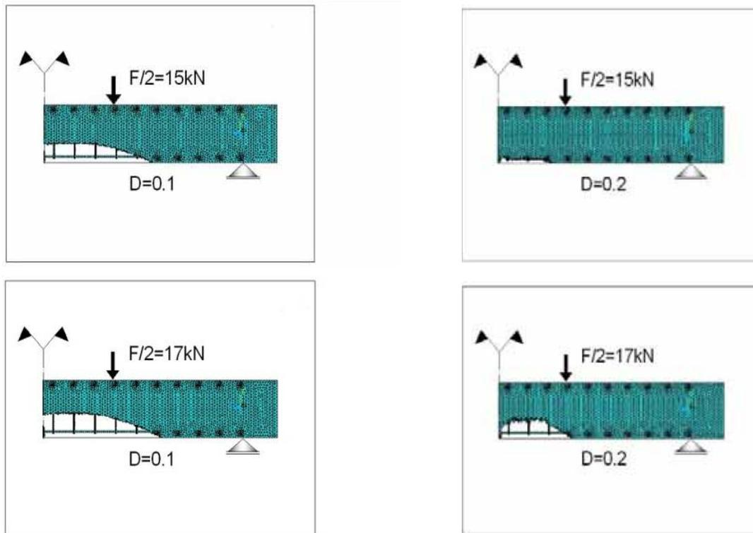
Fig. 5: Initiation and propagation of damaged zones with the applied load increase
