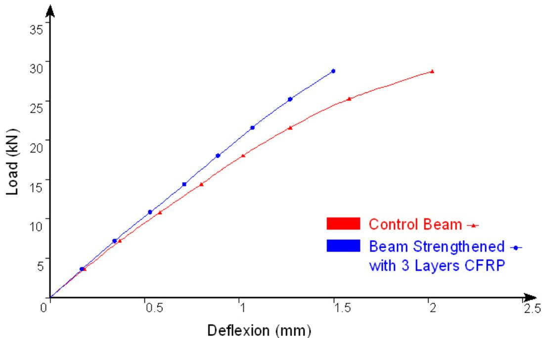
Fig. 7: Gain of rigidity after casting 3 layers CFRP
