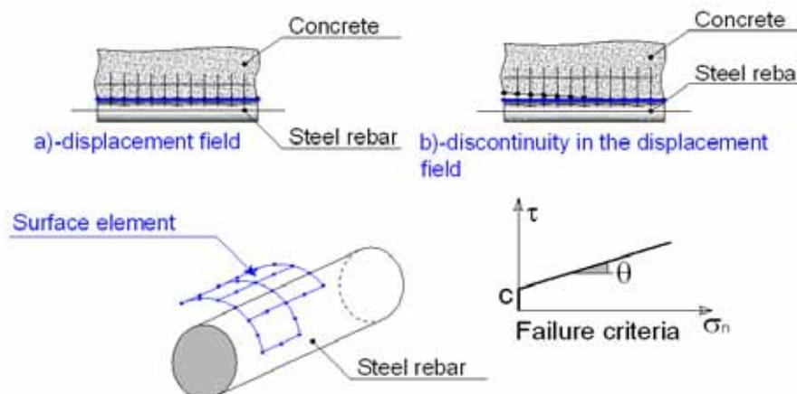
Fig. 3: Concrete interface
