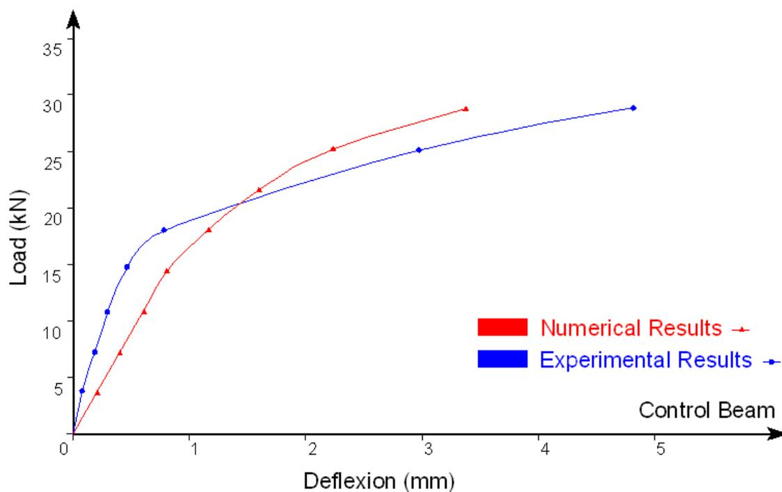
Fig. 6: Comparison between the experimentally and numerically obtained load- deflection beam response
