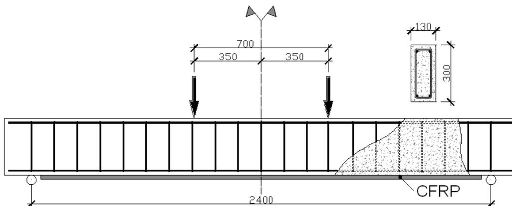
Fig. 2: Reinforced Concrete Beam Geometry
