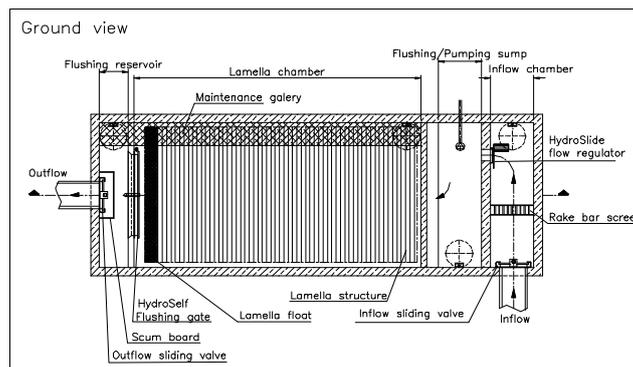
Figure 2. Functional diagram HydroM.E.S.I. Lamella separator, overview.
