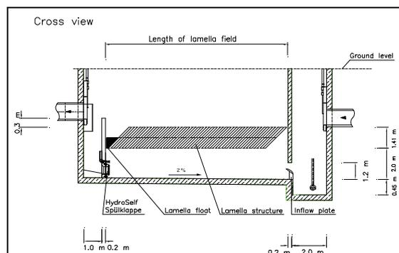
Figure 4. Standard tank design for HydroM.E.S.I. particle separator
