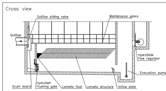
Figure 3. Functional diagram HydroM.E.S.I. Lamella separator, cross view.
