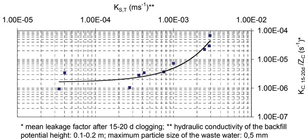
Figure 1: Leakage factor ( $K_C/Z_C$ ) and conductivity of the backfill
