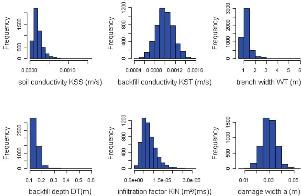
Figure 3: Structural Input data of the Monte-Carlo-Simulations
