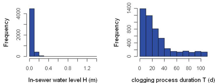
Figure 4: Distribution of input parameters, which influence the dynamics of the exfiltration process.
