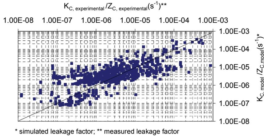
Figure 2: Measured and simulated leakage factors
