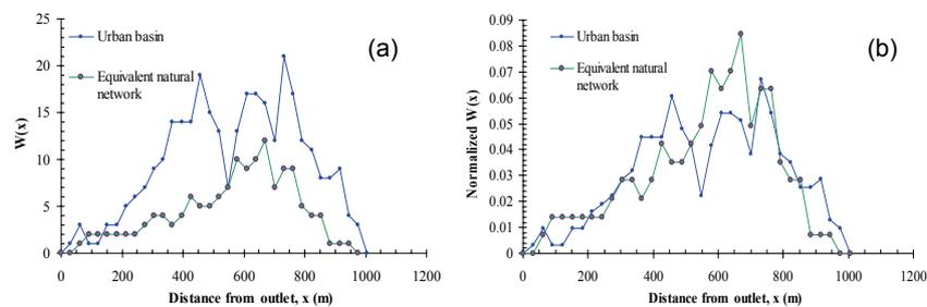
Figure 1. Width functions for pre- and post-development conditions: (a) Comparison of the width functions, (b) Comparison of the normalized width functions.
