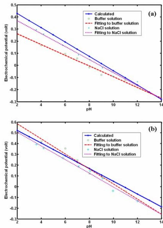
Fig. 3. Electrochemical potential vs.  $pH$  comparison curves between calculated and experimental measurements fitted to a linear equation for  $ZnO$  nanorods grown on (a) plane and (b) 2DMPPS  $n-Si$  substrates immersed in buffer and  $NaCl$  solutions.
